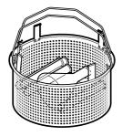
If the containers are placed with their openings facing upward, it is hard for air to sufficiently escape from the container and for steam to sufficiently penetrate inside, thus resulting in incomplete sterilization.
