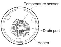
(Plan of bottom of chamber inside)
