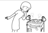
Since high-temperature steam will escape when the cover is opened, wait until the steam dissipates. During this time, keep your head away from the product.
