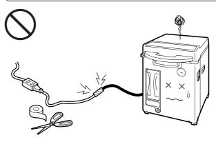
Do not connect the power cord or plug to an extension cord.
