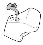
2) Pour water up to the LOW (minimum) level mark, insert the packings to the holes of the product and connect the exhaust hoses.
