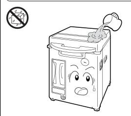
Failure to observe this caution may cause short-circuits in live parts, resulting in electric shock or fire.
