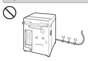
Failure to observe this caution may overheat the power cord, resulting in fire.
