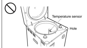
Failure to observe this warning may destabilize control of the product or result in incomplete sterilization.
