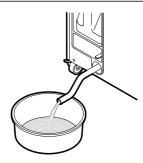
Insert the attached drain hose in the drain water port and drain water at least 2 hours after operation. If water is drained out in haste, hot water may splatter, resulting in burns or damage to the floor. Repeated use of the same heating water may corrode the chamber or clog the piping.
