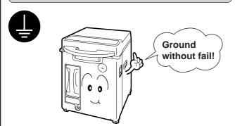
Make sure that the product has been properly grounded. Be sure to connect one end of grounding line to the ground and the other end to the grounding terminal.
