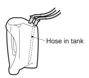
Be sure to insert the hose in the tank into the holes at the back inside the exhaust tank.
