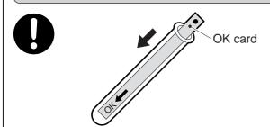
The sterilization performance will vary depending on such factors as the type and volume of objects to be sterilized, the arrangement of objects and the type of container. Therefore, use a sterilization indicator such as an "OK card" for checking the performance.
